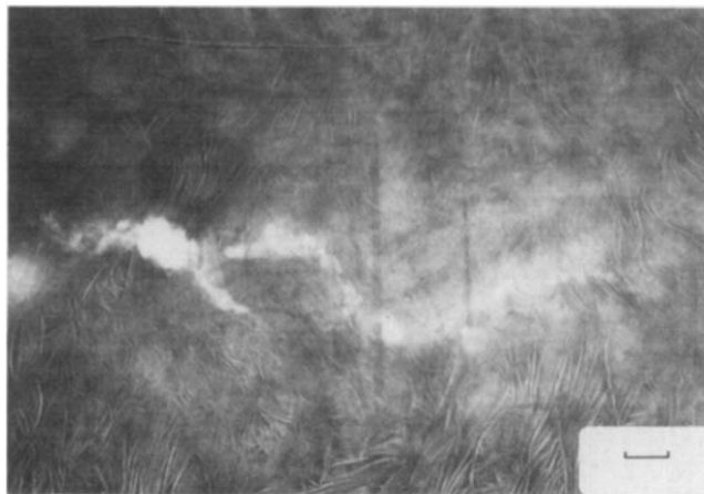
Figure 3 Bright field transmission electron photomicrograph of a dry craze in a spherulite boundary region at the tip of an environmental stress crack in sample F. Marker = 0.33 \mu\text{m}
